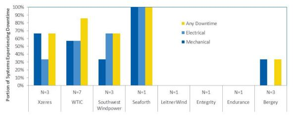
Figure 14. Rates of Reported Downtime by Failure Type and Turbine Manufacturer
