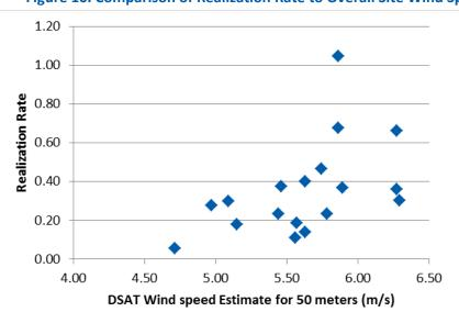
Figure 10. Comparison of Realization Rate to Overall Site Wind Speed
