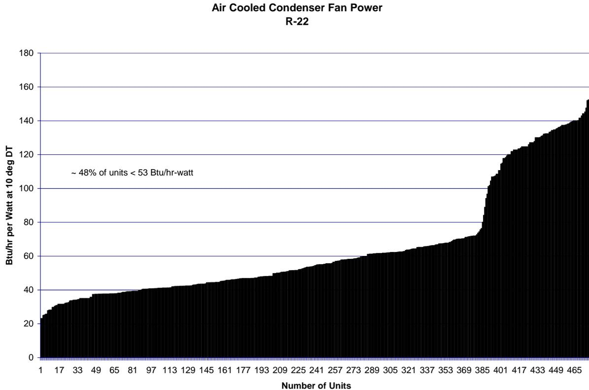
*Figure 5 Air Cooled Condenser Specific Fan Power Distribution*
