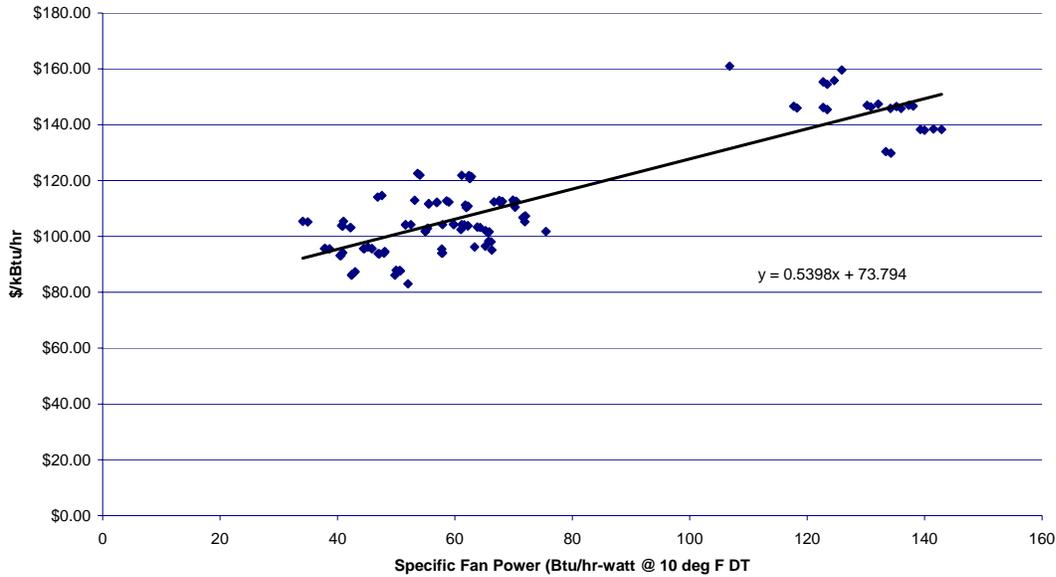
*Figure 8 Air Cooled Condenser Cost Correlation*
