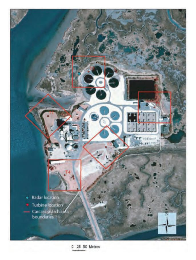
Figure 4. Atlantic City Utilities Authority (ACUA) study site showing the location of five wind turbines, carcass search area boundaries and location of dual marine radar system. Turbine (T) locations are numbered 1-5.
