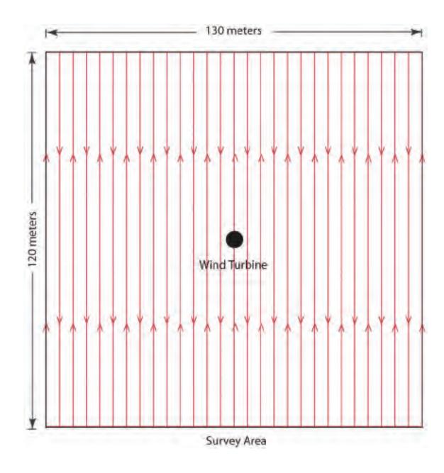
Figure 5. Schematic of the transect layout for carcass search surveys. Transects are spaced approximately 5 meters apart. The survey plot is oriented to maximize the searchable area. While walking each transect, the searcher used the unaided eye to conduct the survey, alternately scanning an area that extended for 2.5 m on either side of his/her track.
