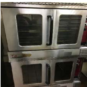
Gas-fired convection oven
