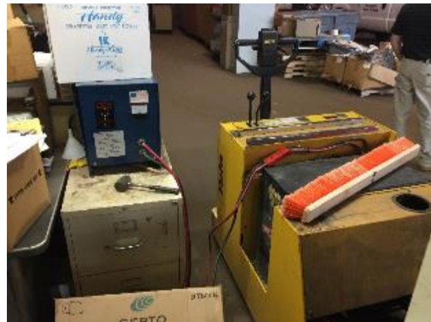
Forklift DC Charger
