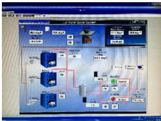
Hot Water Boiler System User Interface
