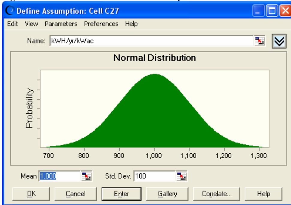
Figure 3-17, Figure 3-18, and Figure 3-19 present the probability distribution for the installed cost of the PV system for each of the project types. PV system costs per kW will vary by installation and location. An analysis of the CORE data indicated that a normal distribution best fit the data. The average system costs from the CORE database were used for the mean value and a standard deviation of 10% was assumed.
