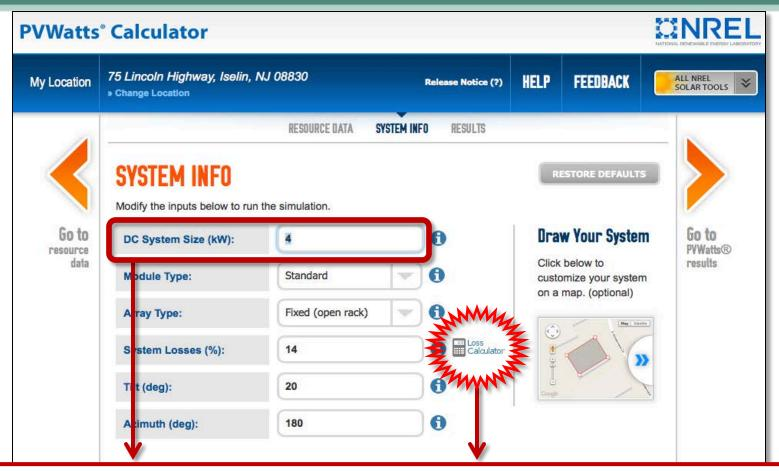
For "Ideal" PVWatts, only change "DC System Size (kW)". All other values remain default. System Losses (%) remains "14". Click on "Loss Calc." to view.
