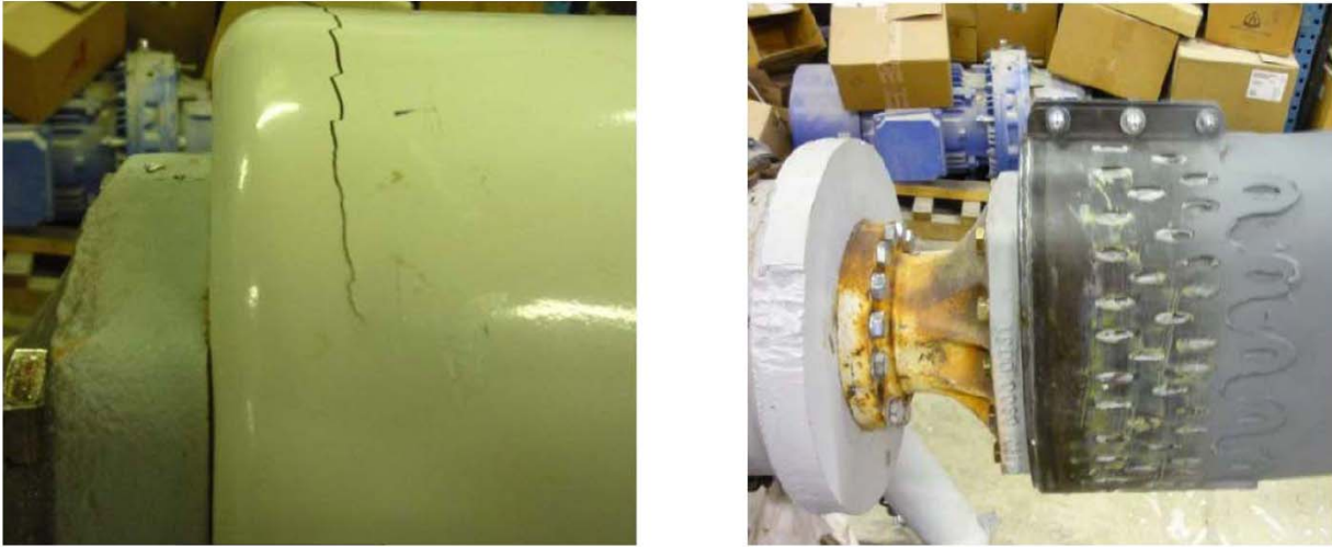
Figure 2. Unbolstered (left) and bolstered (right) root designs
