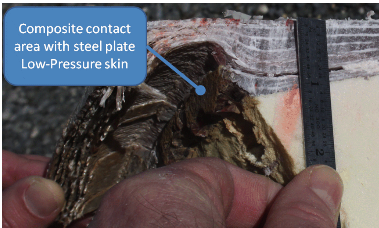
Figure 18. Contact area of composite against steel plate (steel plate missing)
