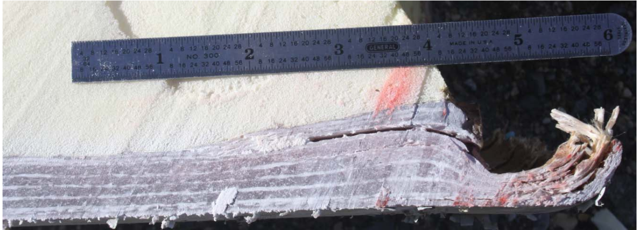
Figure 17. Root-to-tip section of low-pressure skin in the root area
