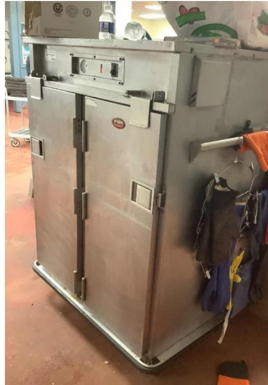
Electric Holding Cabinet
