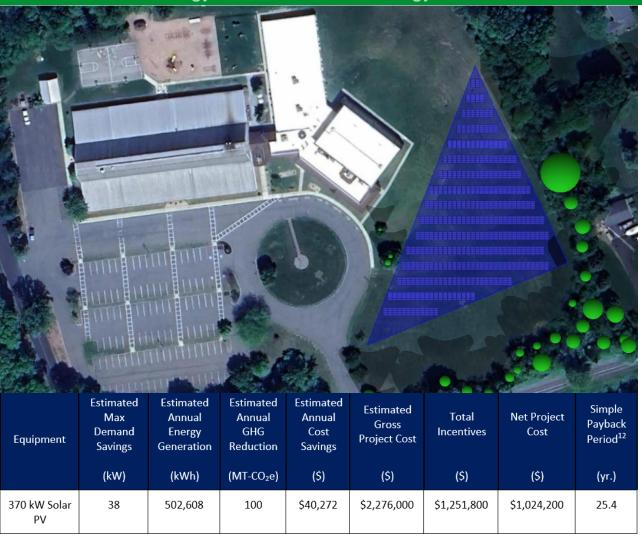
370 kW ground mount Solar PV System: The ground mount solar panels are strategically positioned to make the most efficient use of the open area in front of school, maximizing coverage of the solar energy generation. The projected solar PV system is expected to generate a total energy output of 502,600 kWh, accounting for 100% of the site's total electricity consumption for the year 2023.
