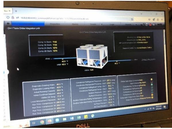
Chiller and BMS Diagram
