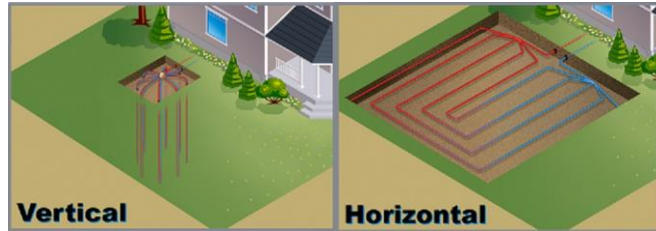
Ground Source Heat Pump (GSHP) (Geothermal)
