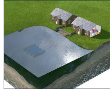
Open-loop, Pond, "Pump and Dump"
