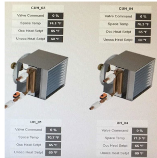
BEMS Screenshot - Hydronic Unit Heaters
