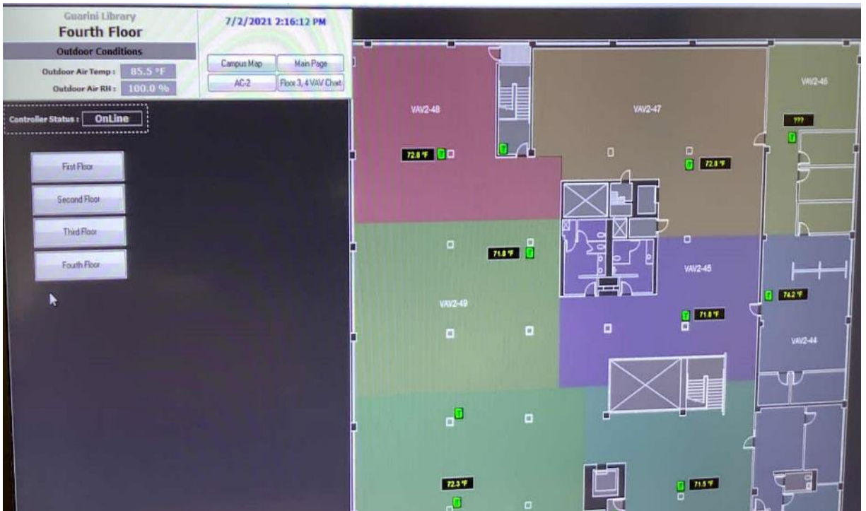
Building Energy Management System for Guarini Library
