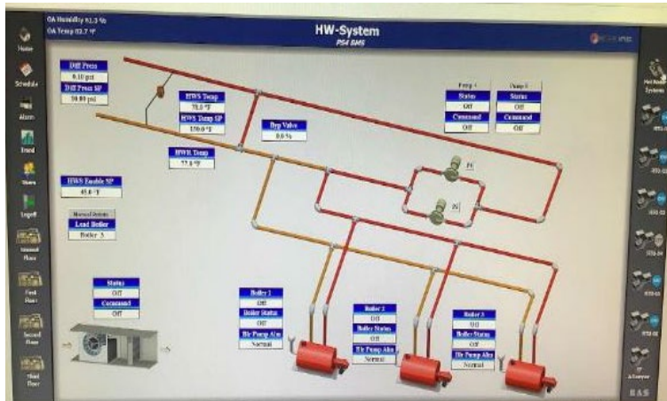
EMS screenshot – Boiler System
