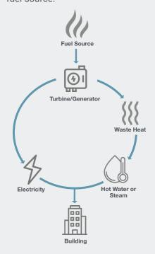
The hot exhaust is recovered and re-used as part of the building's HVAC system, or as steam for manufacturing processes.
